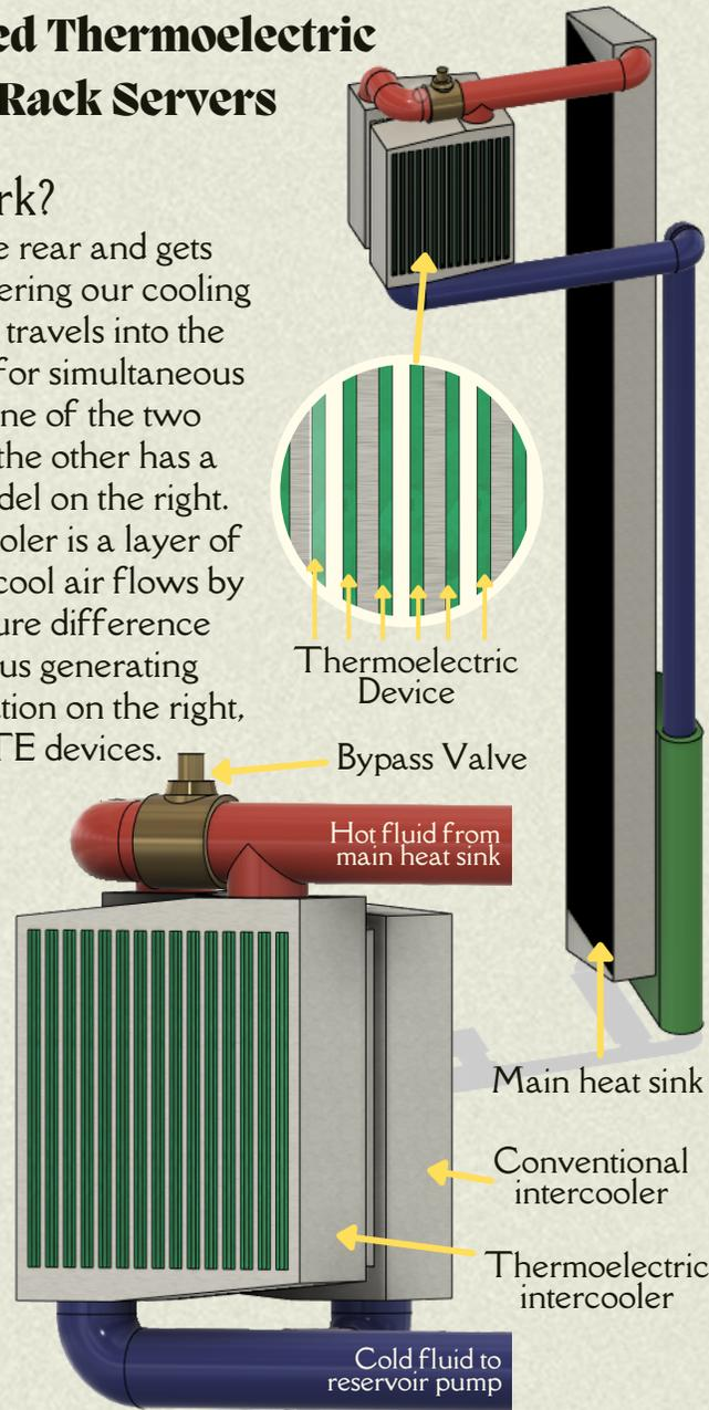
Large data centers usually have arrays of server racks. If our cooling system is installed on multiple racks, airflow can be directed to pass through a line of intercoolers, as illustrated by the model on the left. This localized cooling design, contrary to the traditional method of cooling the entire server room, improves efficiency and is recommended by the U.S. Department of Energy.
